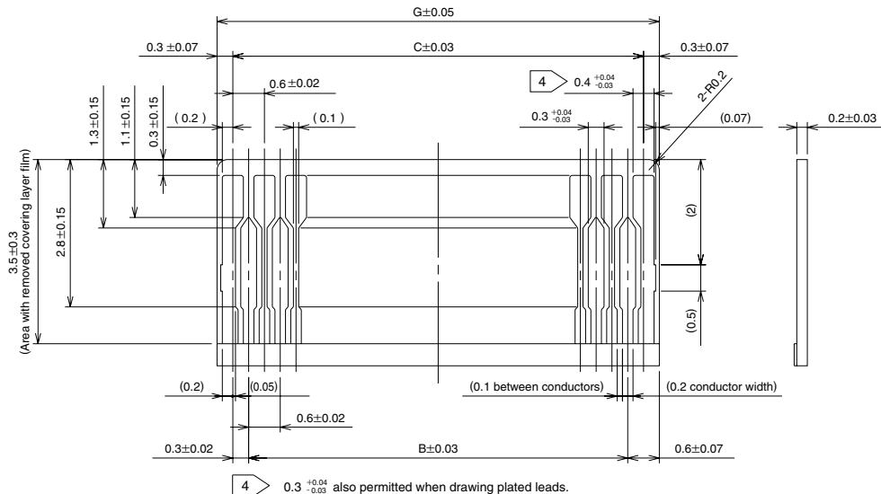
5 Polyamide and thermally hardening adhesive is recommended as the materials for the stiffener.
