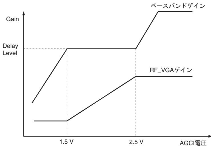
By providing the gain variation shown above, only the baseband block gain is varied during weak input (when the AGCI voltage is high), so the total NF does not worsen. This enables to improve the distortion characteristics by varying only the RF\_VGA circuit gain over the AGCI voltage range of 2.5V to 1.5V.
