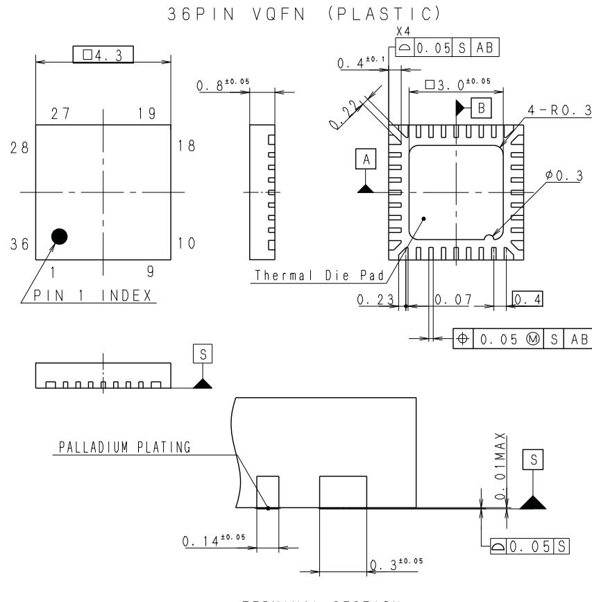
Note: Cutting burr of lead are 0.05mm MAX.
