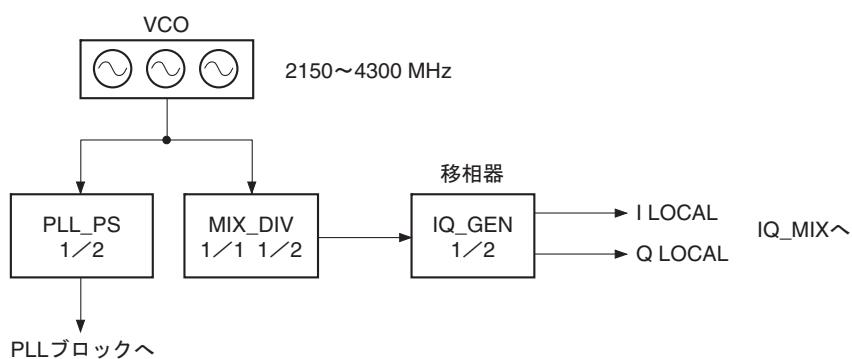
The signal from the VCO is used as the local signal, and is passed through a fixed 1/2 frequency divider and then input to the PLL circuit.
