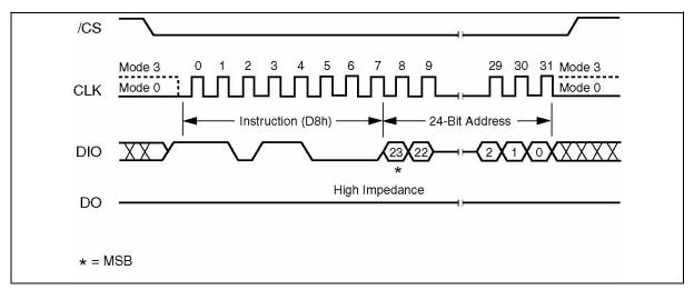
Figure 13. Block Erase Instruction Sequence Diagram
