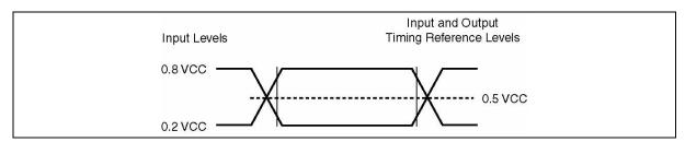
Figure 21. AC Measurement I/O Waveform
