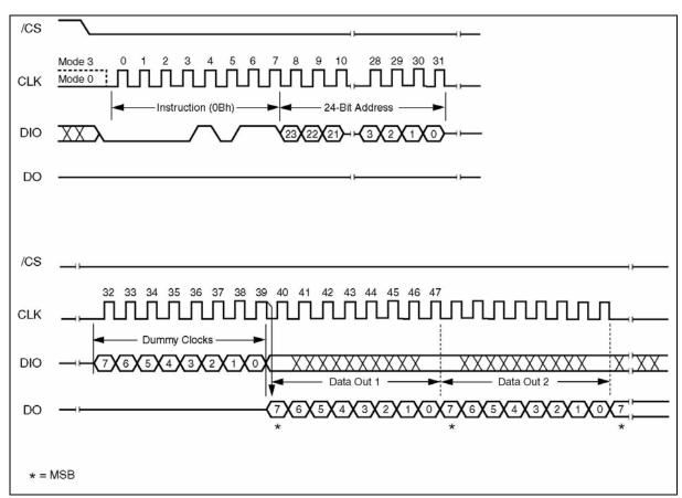
Figure 9. Fast Read Instruction Sequence Diagram
