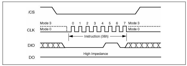
Figure 4. Write Enable Instruction Sequence Diagram
