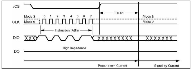
Figure 16. Release Power-down Instruction Sequence
