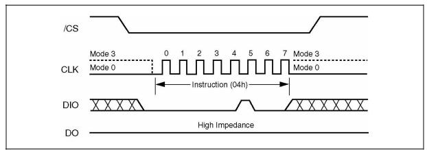
Figure 5. Write Disable Instruction Sequence Diagram
