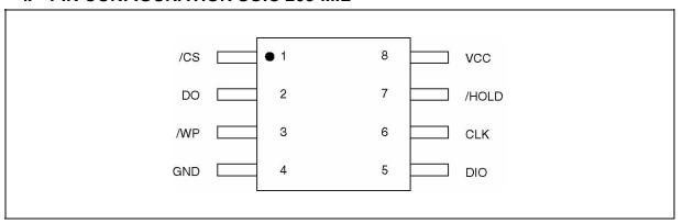
Figure 1b. W25X40 and W25X80 Pin Assignments, 8-pin SOIC (Package Code SS)
