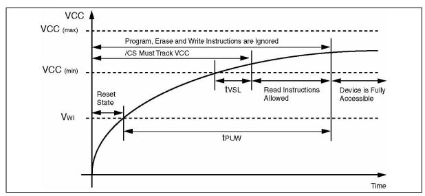
Figure 20. Power-up Timing and Voltage Levels
