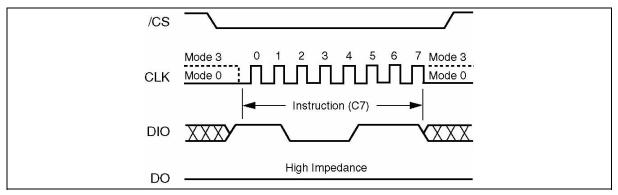
Figure 14. Chip Erase Instruction Sequence Diagram
