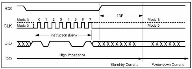
Figure 15. Deep Power-down Instruction Sequence Diagram
