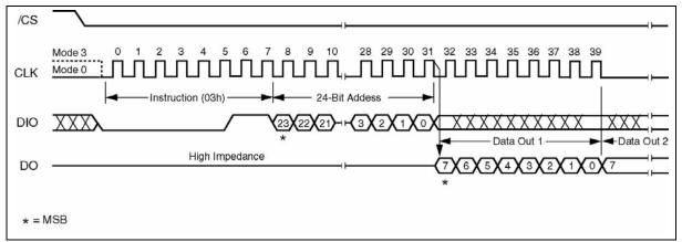
Figure 8. Read Data Instruction Sequence Diagram
