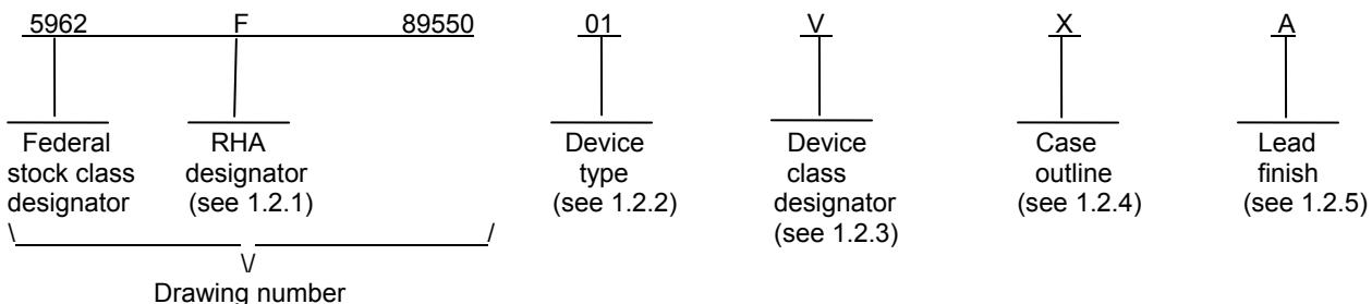
1.2.1 RHA designator. Device classes Q and V RHA marked devices meet the MIL-PRF-38535 specified RHA levels and are marked with the appropriate RHA designator. Device class M RHA marked devices meet the MIL-PRF-38535, appendix A specified RHA levels and are marked with the appropriate RHA designator. A dash (-) indicates a non-RHA device.
