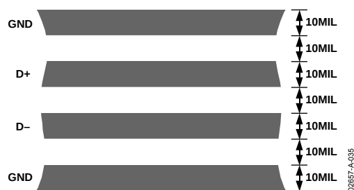
Figure 35. Arrangement of Signal Tracks
