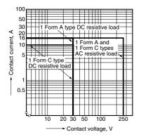
1-(2). Max. switching capacity (2 Form C)
