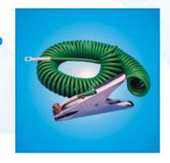
Cen-Stat<sup>™</sup> cable is standard on all Cenlectrex products. Multi-stranded steel conductors for superior mechanical strength combined with Hytrel anti-static coating for optimum chemical and abrasion resistance. With a 1:10 extension ratio Cen-Stat cable is proven to hold its shape after 20,000 continuous extensions.
