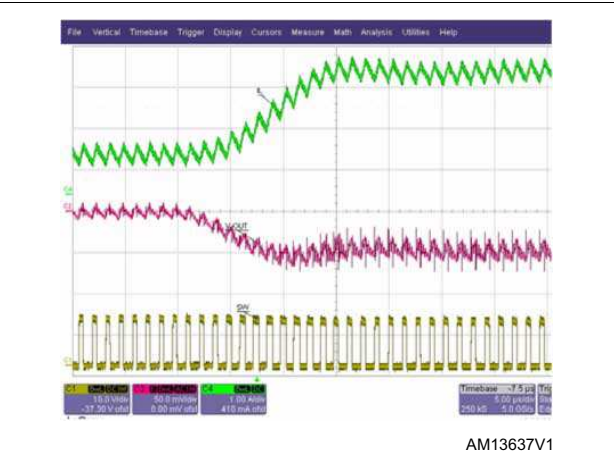
Figure 43. Zoom - 1 A to 3 A load transient ( V_{IN} 12 V)
