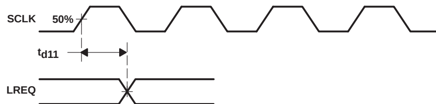
Figure 6-7. TSB12C01A Link-Request-to-Phy-Layer Waveforms
