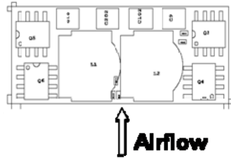
Figure 34. Airflow direction for thermal testing.
