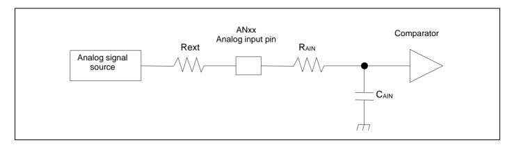
(Equation 1) Ts  $\geq$  ( R<sub>AIN</sub> + Rext )  $\times$  C<sub>AIN</sub>  $\times$  9
