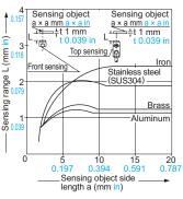
As the sensing object size becomes smaller than the standard size (iron sheet 15 × 15 × t 1 mm 0.591 × 0.591 × t 0.039 in), the sensing range shortens as shown in the left figures.
