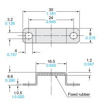
Material: Bracket ... Stainless steel (SUS304) Fixed rubber ... FKM (Fluorine rubber)
