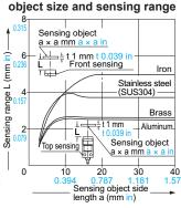
As the sensing object size becomes smaller than the standard size (iron sheet 20 × 20 × t 1 mm 0.787 × 0.787 × t 0.039 in), the sensing range shortens as shown in the left figure.
