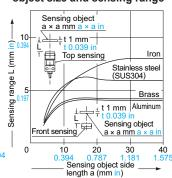
As the sensing object size becomes smaller than the standard size (iron sheet 30 × 30 × t 1 mm 1.181 × 1.181 × t 0.039 in), the sensing range shortens as shown in the left figure.
