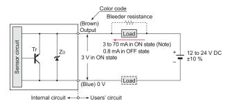
Symbols ... ZD: Surge absorption zener diode Tr: PNP output transistor
