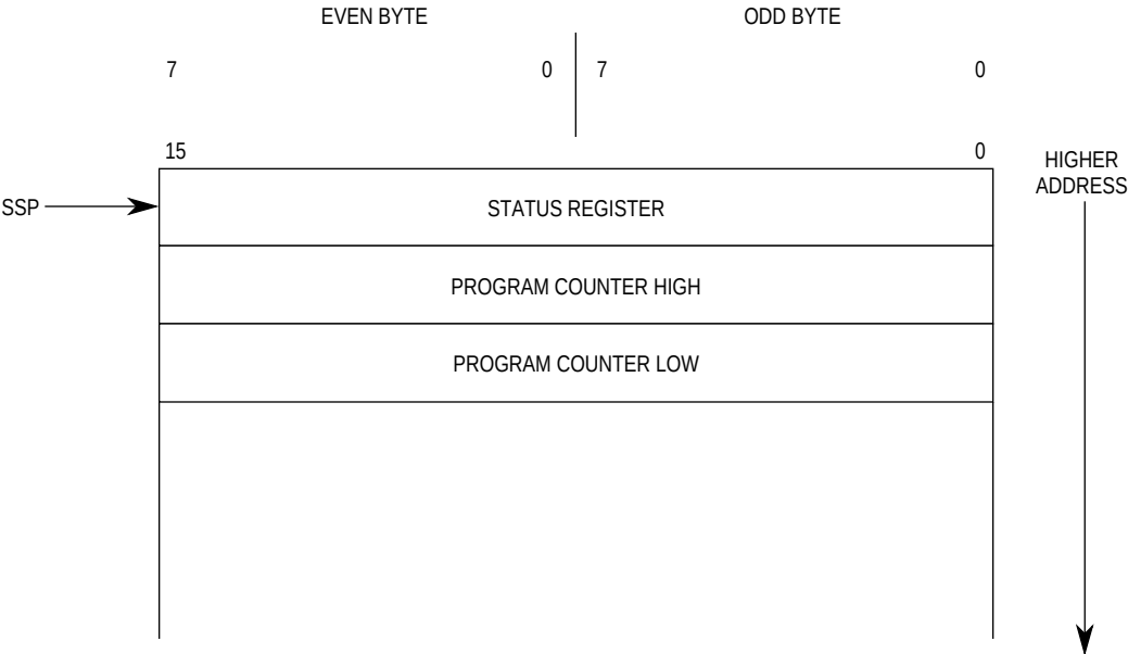
Figure 2-4. M68000 Short-Form Exception Stack Frame
