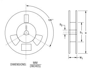
Devices are packed in accordance with EIA standard RS-481-A.
