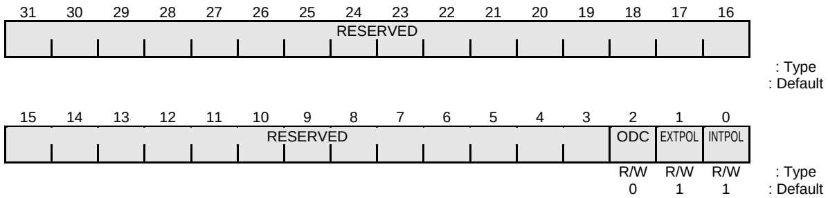
Figure 8-19 Interrupt Request Control Register
