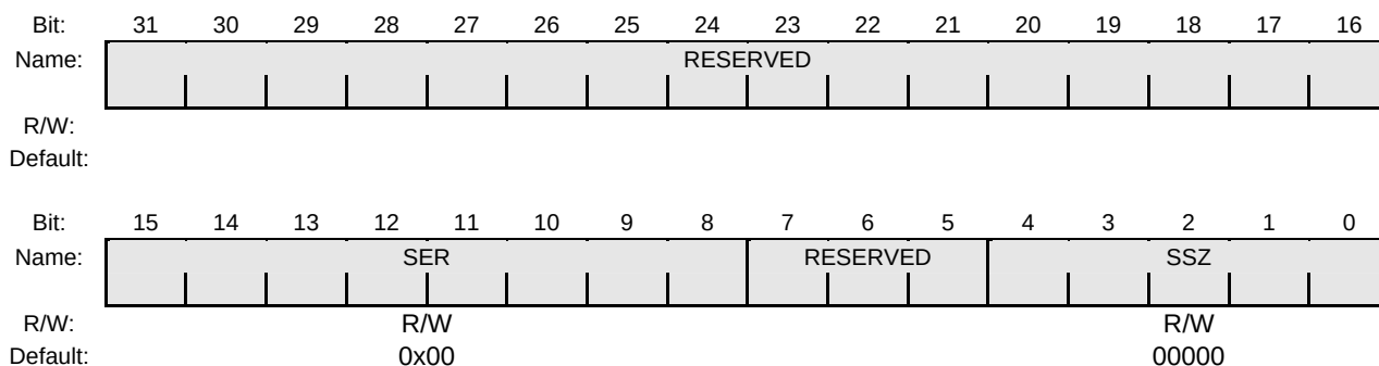
Figure 20-6 SPI Control Register 1 (SPCR1)
