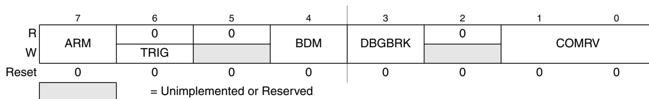
Figure 8-3. Debug Control Register (DBG1)
