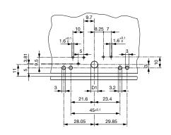
D1 = 6.2 mm mounting from above / D1 = 3.6 mm mounting from below PC Board 1.6 mm / Dimensions without tolerance:  $\leq$  15 =  $\pm$  0.05 / > 15 =  $\pm$  0.10 Drilling diagram CMF6 mirror-inverted
