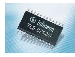
THE TLE 6712G is a 2 loop firing IC specially designed for automotive restraint applications. The device, located in the ECU (Electronic Control Unit) of the airbag system, provides two independent actuator channels for firing loops. Each channel is equipped with various diagnostic functions. Communication between the  $\mu$ C and TLE 6712G is performed via SPI and analog/digital interface pins.
