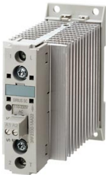
SEMI-COND. CONTACTOR 3RF2,1-PH. AC 51 30 A 40 DEGREES C 24-230 V / 24 V DC SCREW TERMINAL
