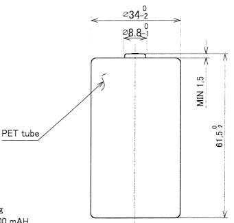
APPROX. WEIGHT: 82 g MINIMUM CAPACITY: 2800 mAH AVERAGE CAPACITY: 3000 mAH
