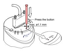
Pror changing the threshold value, push the <ZERO> button and keep it depressed. The threshold keeps changing from the current value (ramp) until the button is released or until the limit of the setting range is reached.
