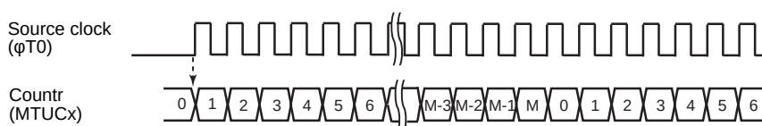
Figure 22-4 Count-up/clear operation when \phi T0 is selected as a source clock
