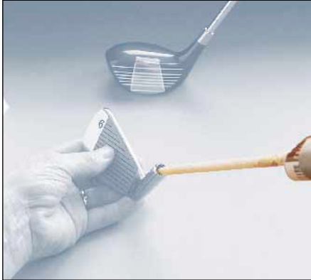
Bonding a golf club head to shaft. 3M Scotch-Weld DP 810
