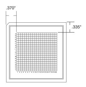
Note: High Accuracy =  $\pm$  - 0.007" registration relative to top/left sides. Must use MicroVu for First Article and In Process Inspections.
