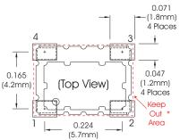
\* Do not route any traces in the keep out area. It is recommended the next layer under the keep out area is to be ground plane.
