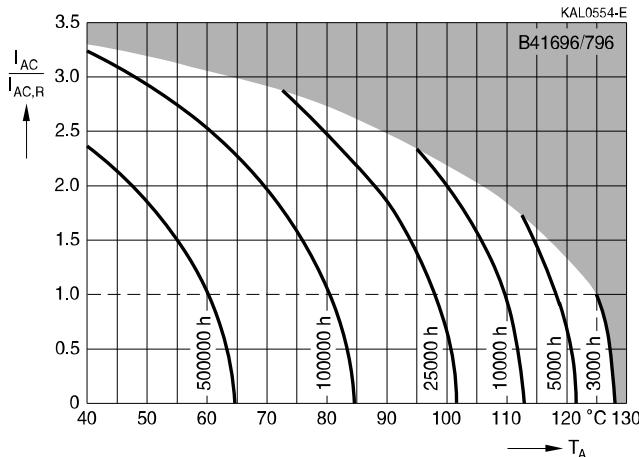
**Useful life<sup>1)</sup>**depending on case temperature  $T_C$  under ripple current operating conditions at  $V_R$
