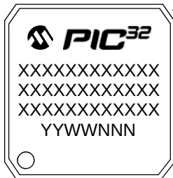
144-Lead TQFP (16x16x1 mm)
