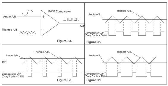
Figures 3a,3b,3c and 3d The audio input Pulse Width Modulates the comparator output.
