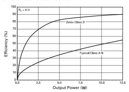
Output Stage Efficiency v Power with  $4\Omega$  and  $8\Omega$  loads
