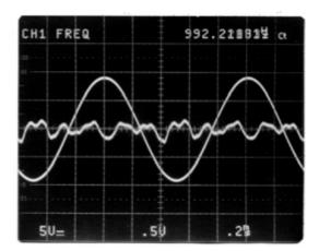
Figure 7a ZETEX Class D Solution. (10W into  $4\Omega$ ) Note lack of Crossover Artifacts
