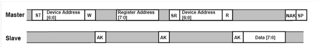
Figure 7. Single Byte Read - The Master is reading one address from the MMA7455L
