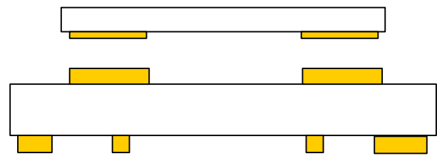
Figure 20. Correct PCB Top Metal Pattern Under Package
