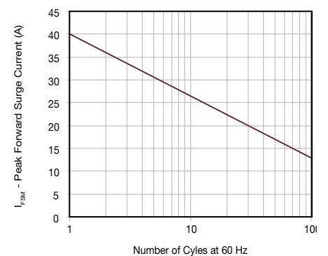
Figure 6 - Maximum Non-Repetitive Forward Surge Current Uni-Directional Only
