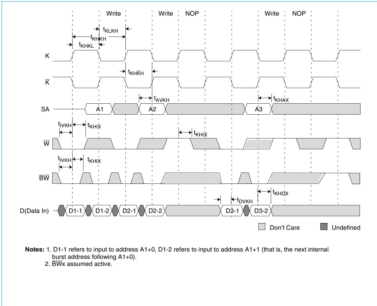
Read, Write, and NOP Timing Diagram
