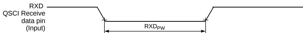
Figure 10-12 RXD Pulse Width
