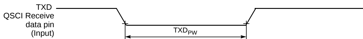
Figure 10-13 TXD Pulse Width
