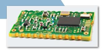
High-performance, long-range radio module with embedded **M-Bus** protocol, for data exchange in stationary and mobile systems between gas, water, heat, electricity meters and concentrators.
