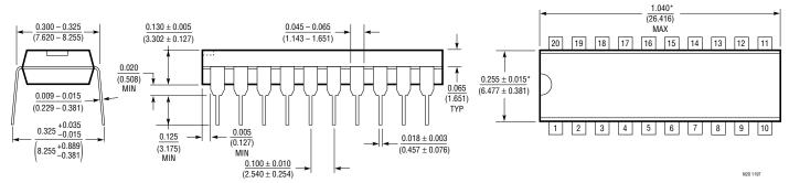
\*THESE DIMENSIONS DO NOT INCLUDE MOLD FLASH OR PROTRUSIONS. MOLD FLASH OR PROTRUSIONS SHALL NOT EXCEED 0.010 INCH (0.254mm)
