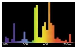
Of all the LUMILUX® lamps, the colour version LUMILUX INTERNA® comes closest to the warm light of an incandescent lamp. With a colour temperature of 2700 K, it gives its surroundings a feeling of homeliness and comfort. Wood, for instance, is highlighted particularly strongly by the light colour LUMILUX INTERNA®; this makes it ideal for use inside furniture and for indirect lighting.
