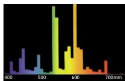
LUMILUX® Warm White is the ideal light colour whenever a bright, yet comfortable light is required. This light is perceived as being pleasantly "warm" on account of its colour temperature of 3000 K. It creates a pleasant atmosphere in which to feel comfortable.
