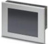
Touch panel with 14.5 cm (5.7") graphics-capable TFT display, 320 x 240 pixels, 1 x Ethernet, 2 x USB, and integrated micro browser
