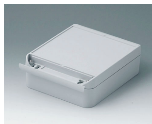
C6015181 SMART-BOX WIDTH 5.906" ASA+PC-FR (UL 94 V-0) light gray RAL 7035 7.09"x5.91"x2.36" IP 66
