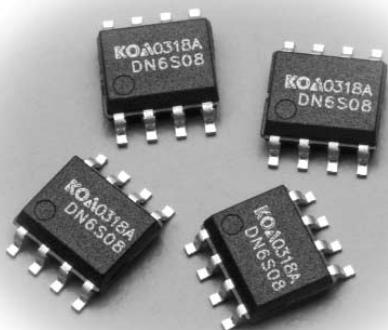
This diode network is designed to provide an integrated solution for the active termination of a single high-speed data signal to eliminate signal undershoot and overshoot. The network has the added benefit of acting to suppress any ESD voltage events by shunting the energy to ground assuring maximum reliability of electronic systems in the field. Trigger levels are defined by the positive and negative bias levels set by the user.
