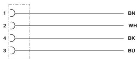
Contact assignment of the M5 socket
