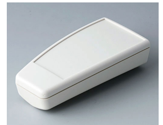
A9066317 SMART-CASE M, Vers. VI ABS (UL 94 HB) off-white RAL 9002 3.78"x1.85"x0.94" IP 40
