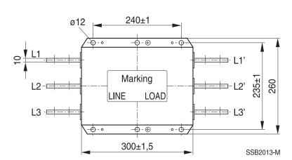
General tolerances according to ISO 2768-cL Dimensions in mm
