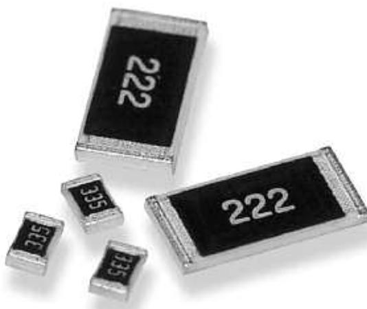
Precious metal terminations are screen printed onto a ceramic base and fired. The resistive element is screen printed and fired and the passivation layer added. Each resistor is trimmed to tolerance by laser. The pre-scribed tile is broken into strips, the end plating is fired on and the strips broken into individual components. Final termination is made by electroplating.
