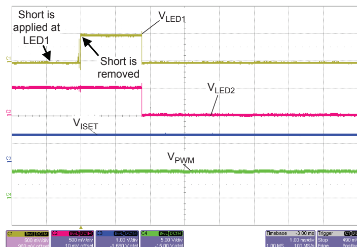
Figure 6: One LED is Shorted to GND.
