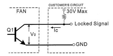
\*Transistor Q1 at "ON" position
