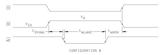
FIGURE 8. Chip clear waveforms.
