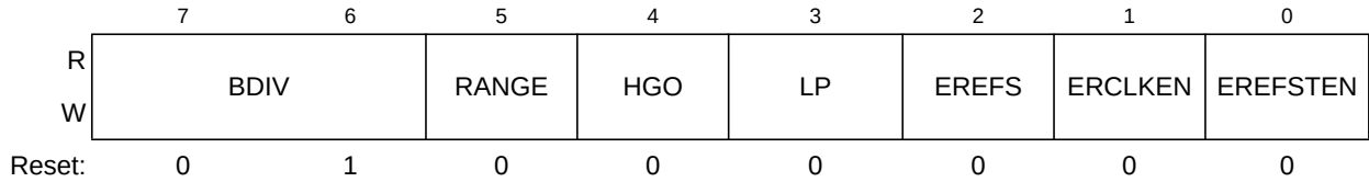
Figure 8-4. MCG Control Register 2 (MCGC2)
