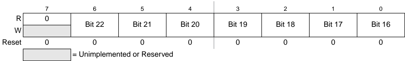
Figure 20-15. Debug Comparator Address High Register (DBGXAH)
