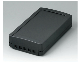
B1075469 TOPTEC 194 F, Vers. II ABS (UL 94 HB) black RAL 9005 7.64"x4.53"x1.81" IP 40
