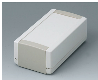
B1060365 TOPTEC 154 H, Vers. I ABS (UL 94 HB) off-white RAL 9002 6.06"x3.31"x2.20" IP 40
