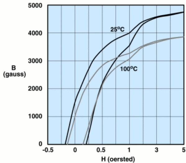
Measured on an 18/10/6mm toroid at 10kHz.
