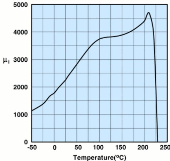
Measured on an 18/10/6mm toroid at 100kHz.
