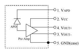
$\frac{\textbf{NOTE}}{\textbf{Under the condition "$V_{APD}$ set, but with $V_{cc}$ absent", optical inputs may result in damage to the TIA. It is necessary to set $V_{cc}$ before optical inputs to prevent such trouble.}$
